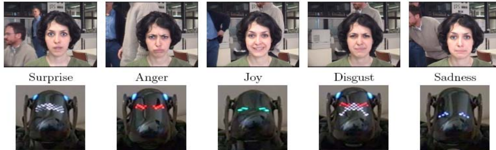
Figure 4. Top: Some detected keyframes associated with the 1600-frame video. Middle: The recognized expression. Bottom: The corresponding robot's response.
