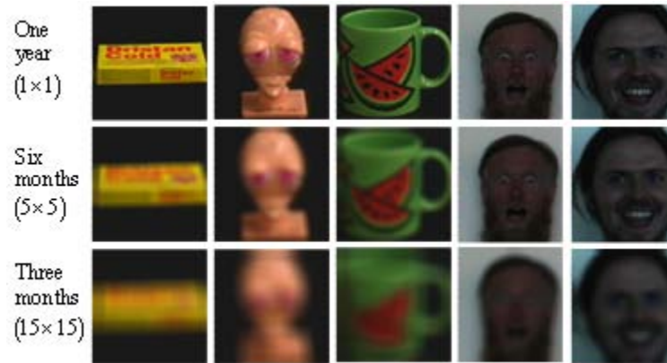
Figure 1. Images filtered with masks of different size. Each group could be associated with different stages of infant vision system.
