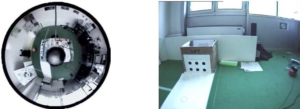
Figure 4. Omnidirectional image (left) and traditional image (right) acquired for a 3D stereo estimation test
