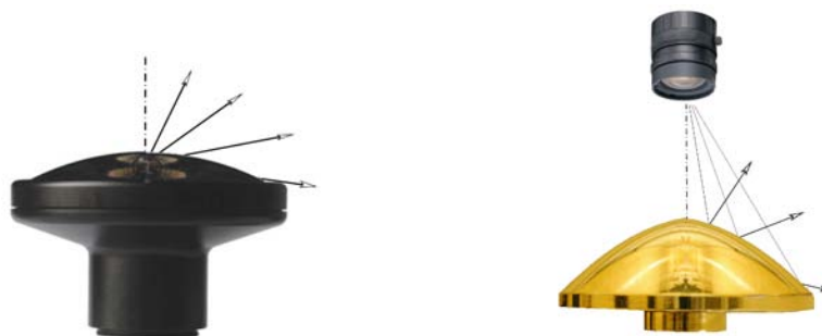
Figure 1. Comparison between image formation in fisheye lenses (left) and catadioptric lenses (right)
